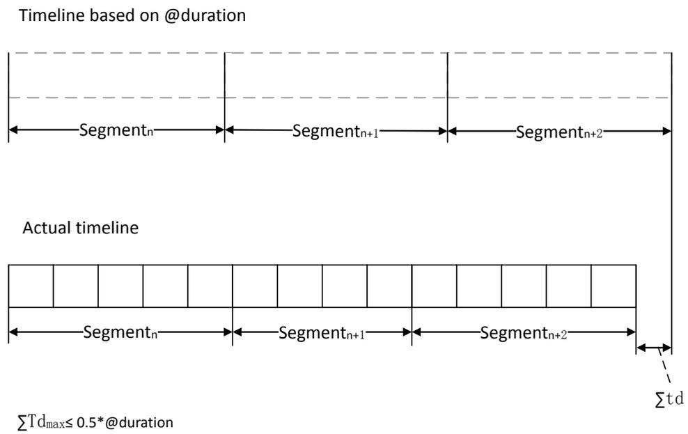
To minimize segment duration fluctuation and meet the preceding constraint, the AC-4 I-frame interval must be at most one fourth of the target segment duration.
