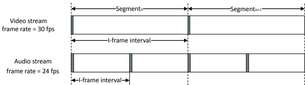
The following figure shows an example where the first I-frames of the video segment<sub>n+1</sub> and audio segment<sub>n+1</sub> are not aligned, and thus this user case is not recommended.
