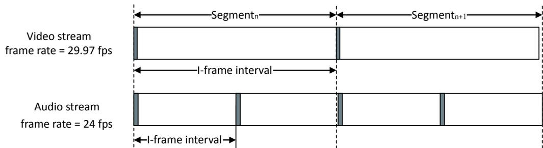
If I-frame alignment cannot be achieved, or if the target segment duration is not an integer multiple of the Dolby AC-4 I-frame interval, Dolby AC-4 segment durations are allowed to fluctuate to maintain close alignment with video segments or the target segment duration timeline. The following figure shows an example where an Dolby AC-4 segment (segment<sub>(n+1)</sub> in the figure) is shorter by one Dolby AC-4 I-frame interval to maintain close segment alignment.
